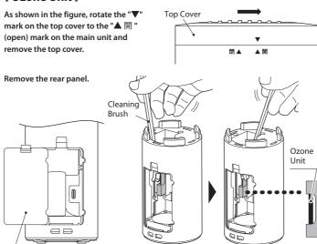
Use a cleaning brush to gently wipe the internal ozone unit from both sides.
