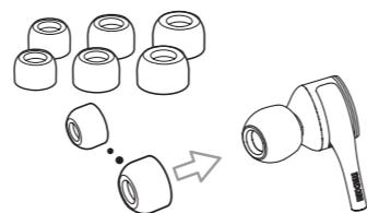
At the time of purchase, size M earpiece are attached to the main unit. If size M does not fit your ears, please replace with the size S or size L earpiece in the contents.
