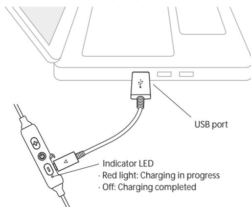
4. Remove the charging USB cable. When the remaining battery power is low, the red indicator light will flash (once every 10 seconds). Please charge immediately.
