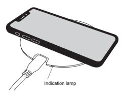
3. When charging is completed, the indication lamp on the main body changes from orange to green. Confirm the indication also on the device to be charged. When charging is completed, remove the device to be charged from the main
