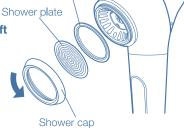
After attaching the washer to the main unit, attach the shower plate over the washer and turn the shower cap clockwise until it is securely installed.
