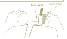
Remove dust from the rear case and main unit using a brush or vacuum cleaner.
